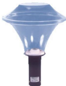
**LUMINAIRE:** Comprises a control gear capsule diecast from Lm6 aluminium alloy. It is fitted with a VPIT copper ballast, CFL lamp holders and mains connector. A clear acrylic diffuser is screwed on top of the capsule.
