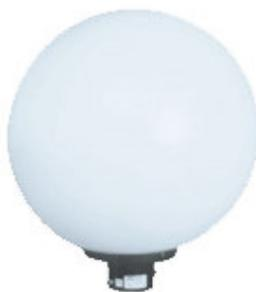
**LUMINAIRE:** Comprises a control gear capsule diecast from LM6 aluminium alloy. It is fitted with a copper wound polyester ballast, lamp holder and mains connector. A rotational moulded spherical diffuser of polyethylene is fixed on top of the capsule. The bowl is adequately gasketed for weather proofness.
