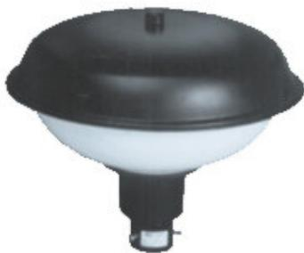
**LUMINAIRE:** Comprises a control gear capsule diecast from LM6 aluminium alloy. It is fitted with a copper wound polyester ballast, lamp holder and mains connector. An opal diffuser, spun aluminium canopy and gasket are assembled over the capsule and held in position with zinc plated brackets and a knurl headed knob. Capsule and canopy have stove enamel mat black finish from outside. Inner surface of canopy has reflector white stove enamel finish.
