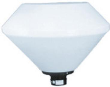
**LUMINAIRE:** Comprises a control gear capsule diecast from LM6 aluminium alloy. It is fitted with a copper wound polyester ballast, lamp holder and mains connector. A rotational moulded diffuser of polyethylene is screwed on top of the capsule. The diffuser is adequately gasketed for weather proofness.
