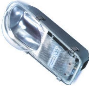
**LUMINAIRE:** Comprises a single piece die cast aluminum LM6 housing in stove enamel hammer tone grey finish from outside. An elegantly shaped high transparency clear acrylic cover is held in position by stainless steel toggles. The control gear compartment is prewired with copper wound polyester ballast, power factor improvement capacitor, electronic ignitor and mains connector. A synthetic rubber gasket prevents insects entry inside the housing.
