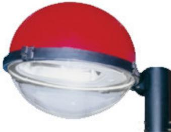
**LUMINAIRE:** Comprises a diecast LM6 aluminium rim which holds the POT (precision optics technology) reflector, gear tray, spun aluminium top bowl, clear acrylic bottom bowl and mounting pipe. Luminaire is prewired with copper wound polyester ballast, power factor improvement capacitor, electronic ignitor and mains connector. The top bowl is available in choice of colours. Both the bowls are held together by synthetic rubber gasket and toggles making the luminaire dustproof.
