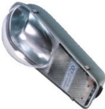
**LUMINAIRE:** Comprises a deep drawn aluminium housing in stove enamel hammertone grey finish. An elegantly shaped high transparency clear acrylic cover is held in position by stainless steel toggles. The control gear housing is prewired with copper wound ballast, power factor improvement capacitor, electronic ignitor and mains connector. A felt gasket impregnated with insecticide prevents entry of insects inside the lamp housing.
