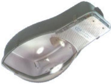
**LUMINAIRE:** Comprises a single piece deep drawn aluminium housing in stove enamel hammer tone grey finish from outside . An elegantly shaped high transparency clear acrylic cover is held in position by stainless steel toggles .The control gear compartment houses a copper wound ballast, power factor improvement capacitor, and mains connector. An electronic ignitor is provided in case of HPSV/MH luminaires. A felt gasket is provided to make the luminaire insect proof and weather proof.
