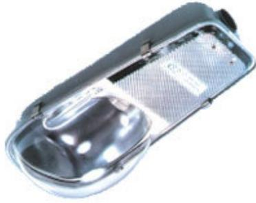
**LUMINAIRE:** Comprises a single piece deep drawn aluminium housing in stove enamel hammertone grey finish. An elegantly shaped high transparency clear acrylic cover is held in position by stainless steel toggles. The control gear compartment is prewired with copper wound polyester ballast, power factor improvement capacitor, electronic ignitor and mains connector. A felt gasket impregnated with insecticide prevents insects entry inside the housing.
