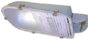
**LUMINAIRE:** Comprises a deep drawn aluminium housing in stove enamel hammertone grey finish. A toughened heat resistant clear glass covering the lamp as well as control gear housing is held in position by stainless steel toggles .The control gear housing is prewired with copper wound ballast, power factor improvement capacitor, electronic ignitor etc. mounted on hingeable gear tray for ease of maintenance . A synthetic rubber gasket ensures high degree of ingress protection.
