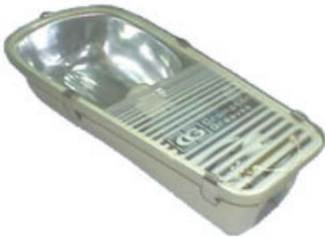
**LUMINAIRE:** Comprises a single piece die cast aluminium LM6 housing in stove enamel hammertone grey finish. An elegantly shaped high transparency clear acrylic cover is held in position by stainless steel toggles. The control gear compartment is prewired with copper wound polyester ballast, power factor improvement capacitor, electronic ignitor and mains connector. A felt gasket impregnated with insecticide prevents insect entry in the housing.
