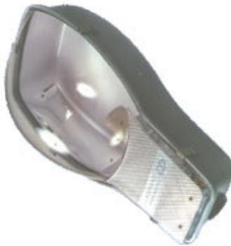
**LUMINAIRE:** Comprises a single piece deep drawn aluminium housing in stove enamel hammer tone grey finish from outside. An elegantly shaped high transparency clear acrylic cover is, held in position by stainless steel toggles. The control gear compartment houses a copper wound ballast, lamp holder, power factor improvement capacitor, electronic ignitor and mains connector. A felt gasket is provided to make the luminaire insect proof and weather proof.
