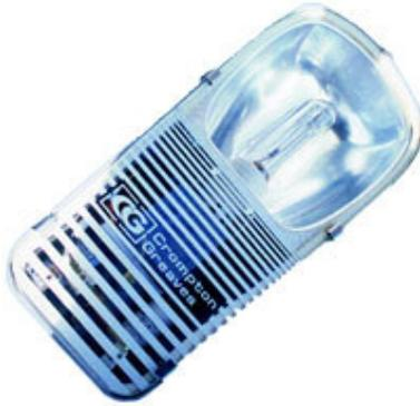
**LUMINAIRE:** Comprises a single piece diecast LM6 aluminium housing in stove enamel grey finish from outside. A toughened heat resistant clear glass covering lamp compartment as well as control gear housing is held in position by stainless steel toggles. Control gear compartment houses a detachable gear tray with a copper wound ballast, power factor improvement capacitor electronic ignitor and mains connector. A synthetic rubber gasket ensures high degree of ingress protection.
