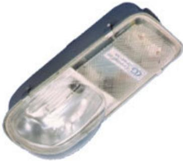
**LUMINAIRE:** Comprises a single piece deep drawn aluminium housing in stove enamel hammertone grey finish from outside. An elegantly shaped high transparency clear acrylic cover is held in position by stainless steel toggles. The control gear compartment is prewired with copper wound polyester ballast, power factor improvement capacitor, electronic ignitor and mains connector. A felt gasket impregnated with insecticide prevents insect entry inside the housing.
