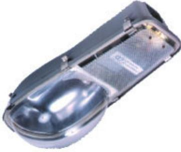
**LUMINAIRE:** Comprises a single piece diecast LM6 aluminium housing in stove enamel grey finish from outside. A toughened heat resistant clear glass covering lamp compartment as well as control gear housing is held in position by stainless steel toggles. Control gear compartment houses a detachable gear tray with a copper wound ballast, power factor improvement capacitor electronic ignitor and mains connector. A synthetic rubber gasket ensures high degree of ingress protection.
