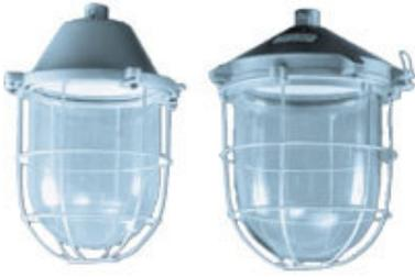
**LUMINAIRE:** I WV12 and I WV11 comprises diecast aluminium LM6 canopy in stove enamel finish. S WV1115 has a diecast aluminium LM6 canopy. A heat resistant well glass with gasket ensures dust/jet proofness. For protection of glass, a galvanized wire guard is provided. Well glass is fitted and adequately gasketed to the canopy by means of retaining clamps.
