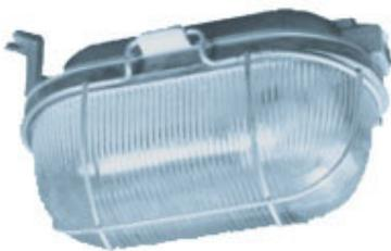
**LUMINAIRE:** Comprises pressure die-cast aluminium LM6 body in stove enamel finish and fitted with a heat resistant elegant glass cover through a gasket. A two pin BC porcelain holder for GLS or a CFL holder is fitted inside the housing. An electro-galvanised MS wire guard ensures protection against pilferage. Glass and wire guard assembly is hinged to the body for ease of maintenance. The CFL bulkhead is prewired with vacuum pressure impregnated copper wound ballast.
