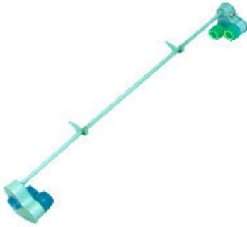
**LUMINAIRE:** Comprises die cast aluminium control gear end boxes connected by means of 19 mm M.S. pipe and finished in hammertone grey. Synthetic rubber gasket is fixed on the periphery of the boxes to make the whole luminaire completely vapour proof. Bi-pin rotor holders are housed in specially designed vapour proof holder casing made of polypropylene. Prewired with vacuum pressure impregnated copper ballasts, power factor improvement capacitor, starters and mains connector.
