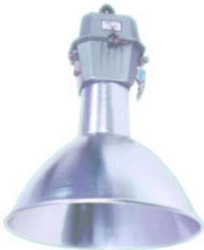
**LUMINAIRE:** Comprises cast aluminium LM6 capsule in stove enamel finish and a spun aluminium reflector. The capsule houses a copper wound ballast, power factor improvement capacitor and mains conenctor. An electronic ignitor is provided in HPSV & MH luminaires. A safety chain is provided on the capsule.
