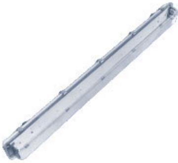
**LUMINAIRE:** Comprises deep drawn CRCA MS sheet housing in white epoxy powder coated finish. Reflector cum control gear tray is fabricated from CRCA MS sheet, finished in stoving white. It is prewired with vacuum pressure impregnated copper wound ballasts, power factor improvement capacitor, push fit type lamp holders and mains connector. An elegantly shaped, high transparency, clear acrylic cover is clamped to the canopy, by stainless steel toggles.
