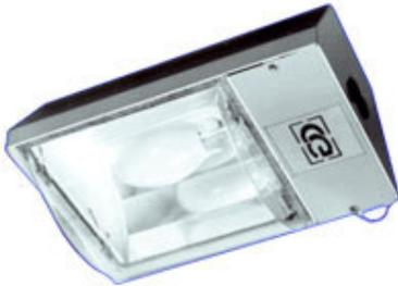
**LUMINAIRE:** Housing fabricated from CRCA MS sheet and finished in stove enamel light grey from outside and white inside. A scientifically designed aluminium reflector ensures optical efficiency. The control gear compartment houses a removable gear tray prewired with a copper wound polyester ballast, power factor improvement capacitor, and mains connector. Lamp compartment is fitted with a high transparency, clear acrylic cover.
