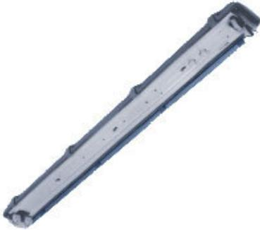
**LUMINAIRE:** Comprises FRP housing in light grey. Reflector plate which also acts as a gear tray, is fabricated from CRCA MS sheet and finished in stove enamel white. It is prewired with vacuum pressure impregnated copper ballast, power factor improvement capacitor, push fit type lamp holders, starters and mains connector. An elegant transparent acrylic cover is clamped to the canopy by toggles.
