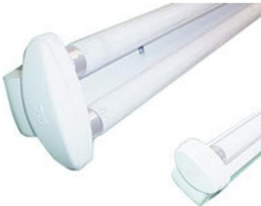
**LUMINAIRE:** Comprises channel fabricated from CRCA MS sheet in stove enamel finish . Channel cover which acts as a reflector is also finished in stove enamel white and has a convenient click fit locking arrangement. Elegantly designed end covers and holder plates of engineering plastic render unique style to the luminaire. It is prewired with vacuum pressure impregnated copper wound ballast, power factor improvement capacitor, pushfit type lamp holders and mains connector.
